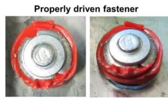
Properly driven fastener A flowering of the top hat seen from top and side views indicates a proper driven X-HSN24 fastener.
